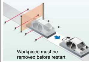
Removal operation required
