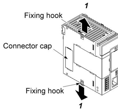
2. Attach unit connectors on the side of each unit.
