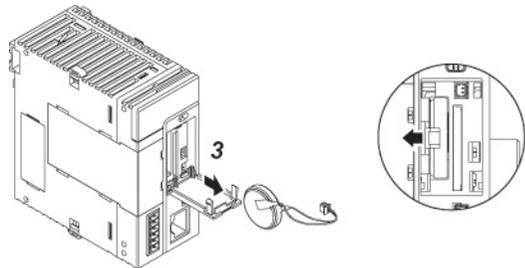
4. While extending the lever to outside, attach a new backup battery to the battery holder.
