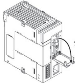
2. Remove the battery connector.
