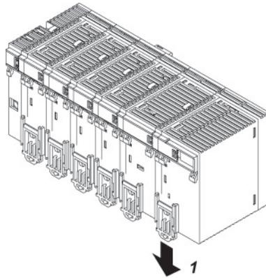
2. Fit the top of the unit attachment part into the DIN rail.
