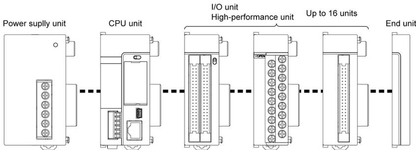
(Note) When the CPU unit is CPS21, a power supply unit cannot be attached.
