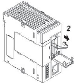
3. While extending the lever to outside, take out the backup battery from the battery holder.
