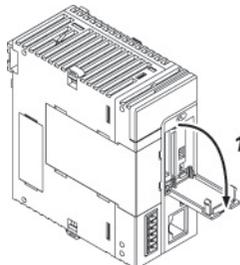
2. Press in an SD memory card into the SD memory card slot until it locks.
