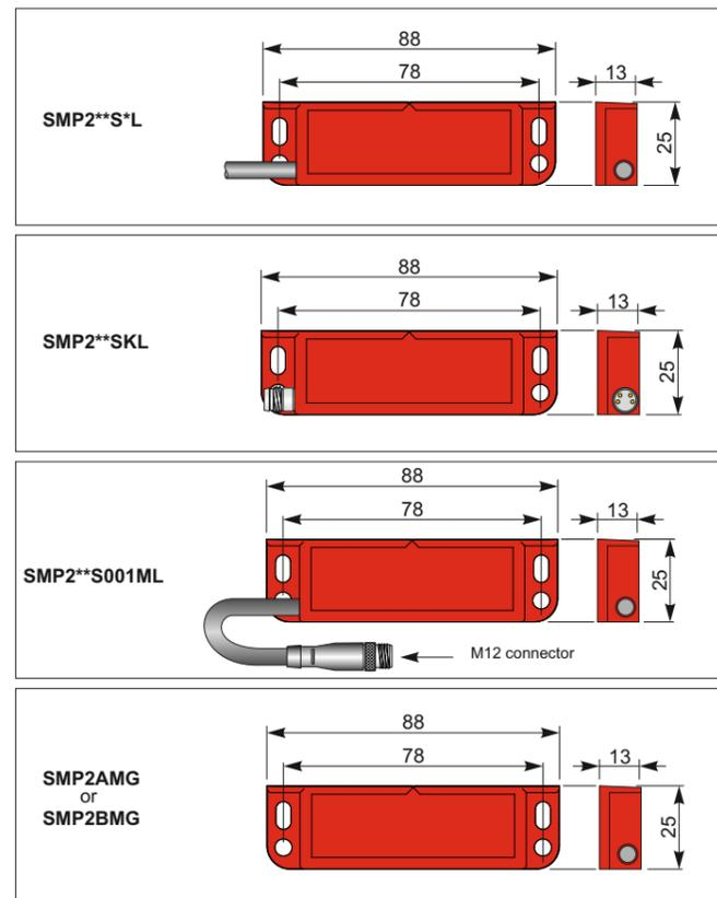
These drawings refer to the sensors with connector or cable exit placed to the left. The models with connection exit placed to the right are mirrored and have the same dimensions..
