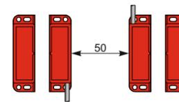
The minimum mounting gap between sensor-actuator systems must be at least 50 mm.
