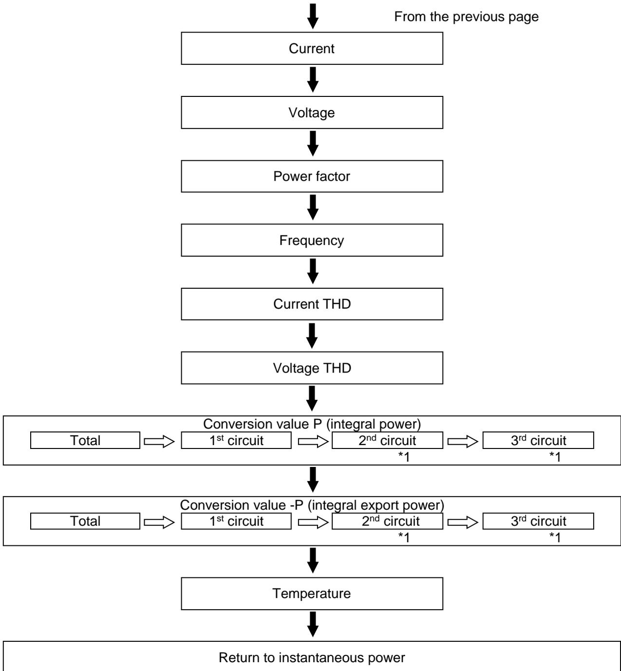
\*1) When 2<sup>nd</sup> circuit and 3<sup>rd</sup> circuit are not measured, [0] are displayed.
