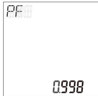
\*Power factor operation is a method assuming balanced load. The error might be big when it measures unbalanced load.
