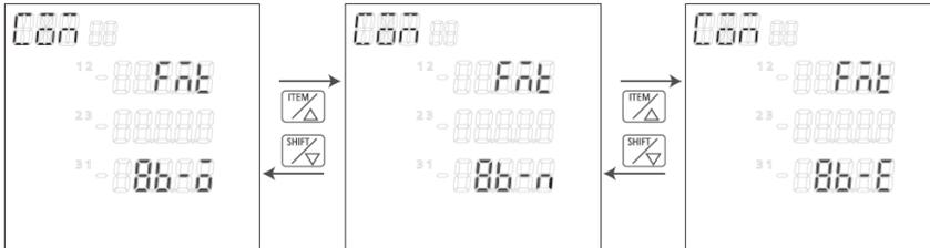
[Set list] 8b-o (8bit odd), 8b-n (8bit none), 8b-E (8bit even) (initial: 8b-o)
