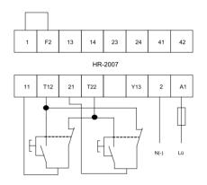
HR-2007 connected to external contactors
