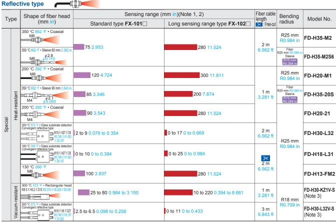
Notes: 1) The sensing range is specified for white non-glossy paper [ $400 \times 400 \text{ mm } 15.748 \times 15.748 \text{ in } (\text{FD-H30-L32, FD-H18-L31}: 50 \times 50 \text{ mm } 1.969 \times 1.969 \text{ in glass substrate, FD-H30-KZ1V-S, FD-H30-L32V-S}: <math>100 \times 100 \times 10.7 \text{ mm } 3.937 \times 3.937 \times 10.028 \text{ in transparent glass)}]$  as the object.
