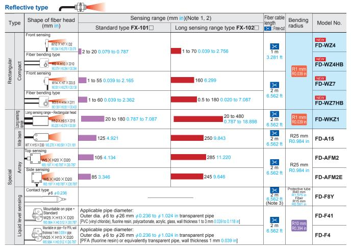
Notes: 1) The sensing range is specified for white non-glossy paper [ $200 \times 200 \text{ mm } 7.874 \times 7.874 \text{ in } (\text{FD-WKZ1}, \text{FD-AFM2E}: 400 \times 400 \text{ mm } 15.478 \times 15.478 \text{ in})$ ] as the object.
