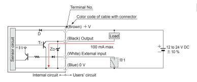
Symbols ... D : Reverse supply polarity protection diode ZD: Surge absorption zener diode Tr : NPN output transistor
