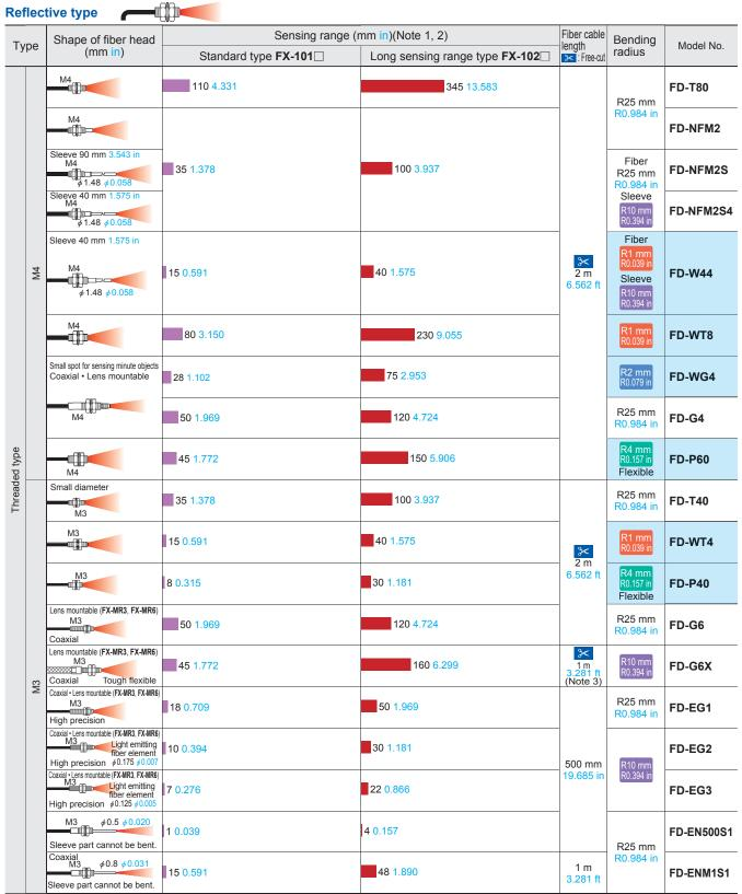
Notes: 1) The sensing range is specified for white non-glossy paper [200×200 mm 7.874×7.874 in (FD-T80, FD-WT8: 400×400 mm 15.748×15.748 in, FD-W44, FD-WT4, FD-P40, FD-G6, FD-EG1, FD-EG3, FD-ER3, FD-EN500S1, FD-ENM1S1: 100×100 mm 3.937×3.937 in)] as the object.
