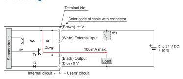
Symbols ... D : Reverse supply polarity protection diode Zb: Surge absorption zener diode Tr : PNP output transistor
