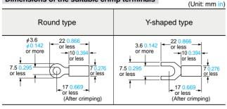
Note: Use crimp terminals with insulating sleeves.
