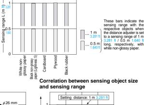
$(200 \times 200 \text{ mm } 7.874 \times 7.874 \text{ in})$  and sensing range
