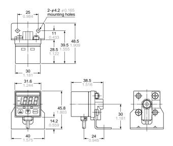
Material: Cold rolled carbon steel (SPCC) (Uni-chrome plated) Two M4 (length 6 mm 0.236 in) pan head screws and two spring washers are attached.
