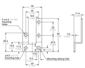
Material: Cold rolled carbon steel (SPCC) (Uni-chrome plated) Two M4 (length 6 mm 0.236 in) pan head screws and two spring washers are attached.
