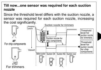
In case of DP3...operation efficiency UP! Since the threshold level can be automatically changed by the auto-reference function, two suction nozzles can be used, alternately, with one sensor.
