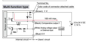
Symbols ...  $D_1$ ,  $D_2$ : Reverse supply polarity protection diode
