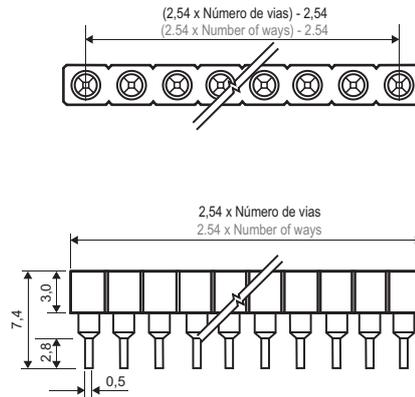
Tolerâncias / Tolerance:  $\pm 0,20\text{mm}$
