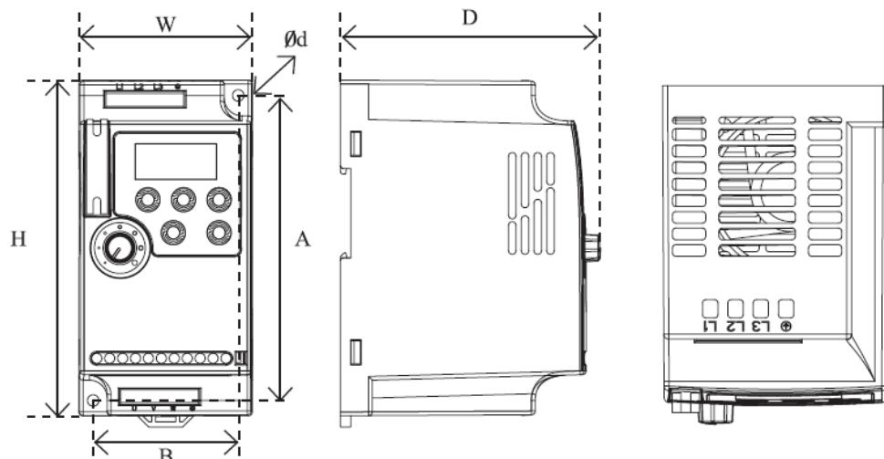
Note: Support for standard 35mm rail mounting(below 5.5kW)
